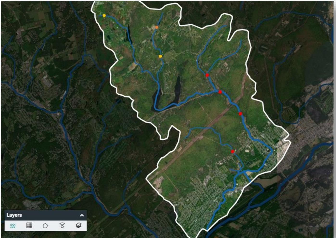
**Figure 26.** Culverts in the Abraham's watershed in need of replacement. Yellow indicates minor barrier to aquatic organisms, orange indicates moderate barrier to aquatic organisms, and red indicates severe barriers to aquatic organisms.
