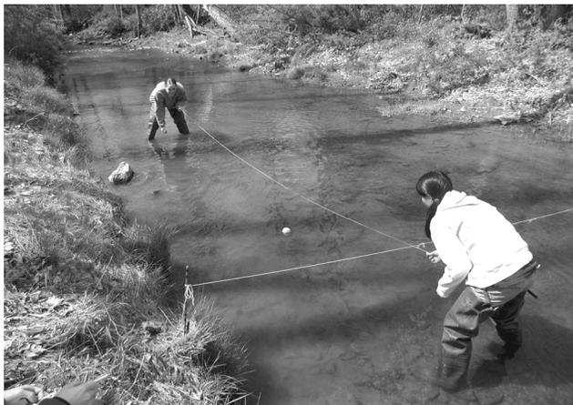
Stephanie Serrano and Samantha Fisher measure the velocity of the stream by measuring how long it takes a tennis ball to travel 30 meters.
