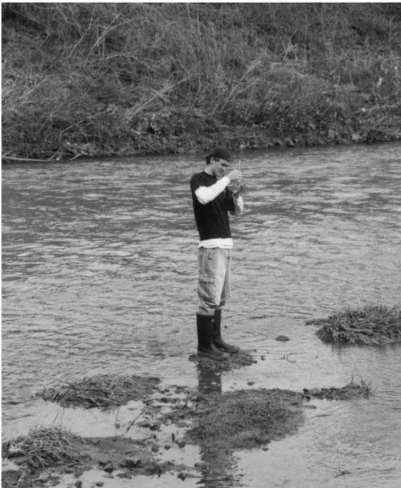
Andy Villa uses a simple thermometer to read the stream temperature.
