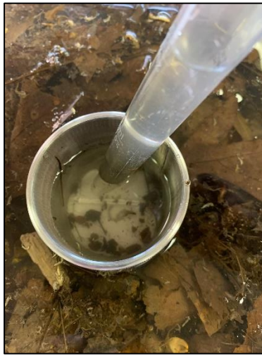
Photos 10-12. Contents of the subsampling grid are removed using spoons, turkey basters, etc.
