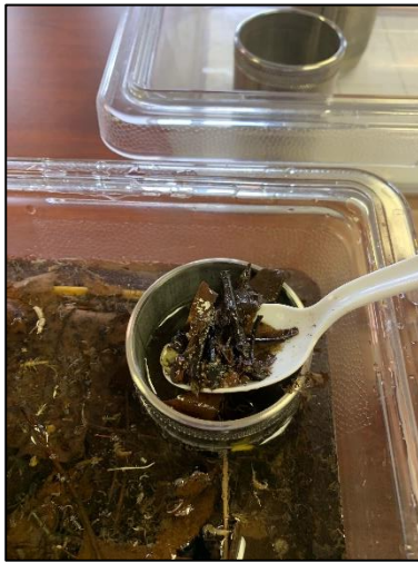
Photos 10-12. Contents of the subsampling grid are removed using spoons, turkey basters, etc.
