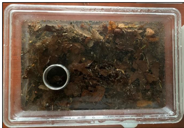
Photo 9. Subsampling pan with sample contents and one “cookie cutter” grid selected.
